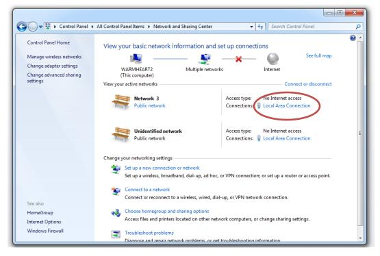
The procedure for assigning an IP address manually varies by computer operating system but they all have the same basic information. In Windows7, go to Control Panel and then go to the Network and Sharing Center. Find the blue "Local Area Connection" link and click on it.
