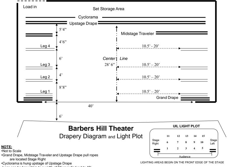
•Legs can be brought in to a width of 21' or pulled out to 40'
