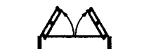
4.2.2.6 - FLAT WITH CASEMENT WINDOW (SHOW MUNTINS AND MULLIONS OF WINDOW AS DESIGNED)
