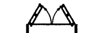
4.2.2.6 - FLAT WITH CASEMENT WINDOW (SHOW MUNTINS AND MULLIONS OF WINDOW AS DESIGNED)
