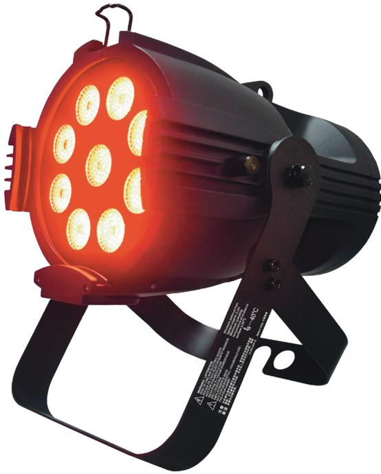
The SL PAR 155 ZOOM is a die-cast aluminum LED Par can that utilizes nine homogenized RGBW LEDs to produce over 3200 lumens of output. The manual zoom provides a beam angle range from 8° to 40° and the split yoke bracket allows for easy hanging or floor mounting.
